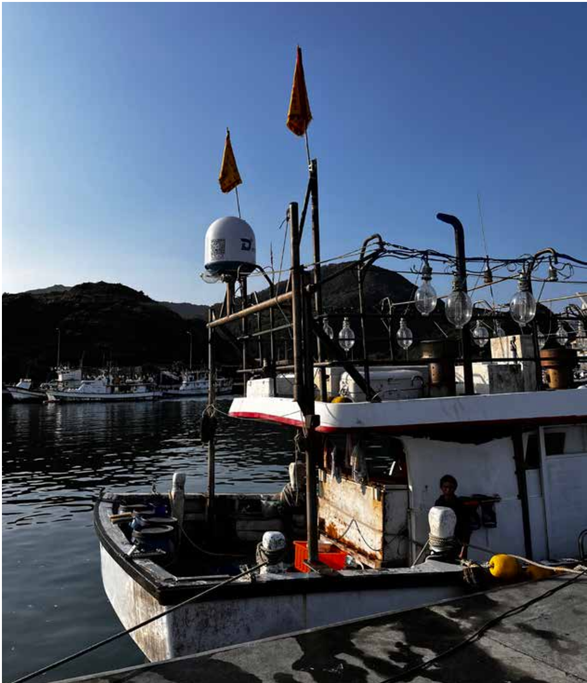
A Taiwanese fishing vessel with a visible device installed for using satellite Wi-Fi
